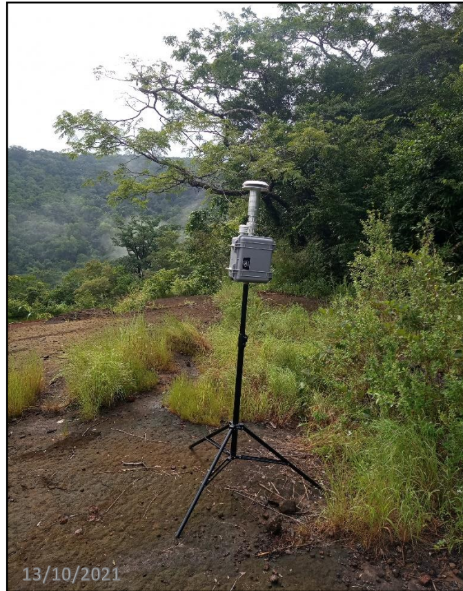
Plate 1: ARA N-FRM Sampler PM 2.5 Setup and monitoring at Tacugama site
