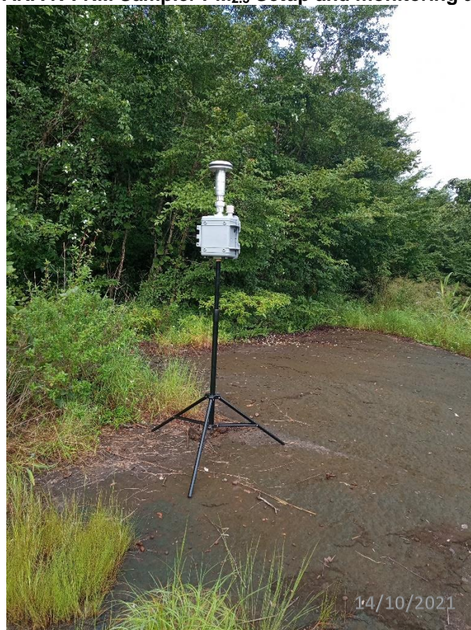
Plate 2: ARA N-FRM Sampler PM 10 Setup and monitoring at Tacugama site.
