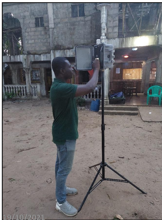
Plate 1: ARA N-FRM Sampler \text{PM}_{10} Setup and monitoring at River No.2
