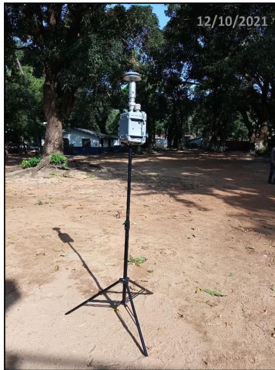
Plate 2: ARA N-FRM Sampler PM 2.5 Setup and monitoring at River No.2
