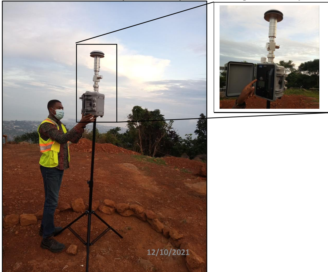
Plate 2: ARA N-FRM Sampler PM 2.5 Setup and monitoring at Leicester peak
