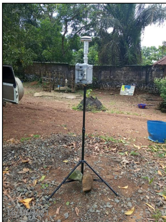
Plate 2: ARA N-FRM Sampler PM 2.5 Setup and monitoring at Bureh Beach
