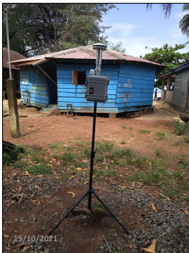
Plate 1: ARA N-FRM Sampler PM 10 Setup and monitoring at Bureh Beach
