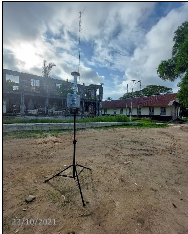
Plate 1: ARA N-FRM Sampler PM 10 Setup and monitoring at Bonthe
