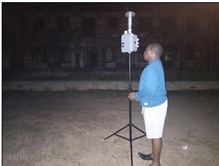
Plate 2: ARA N-FRM Sampler PM 2.5 Setup and monitoring at Bonthe
